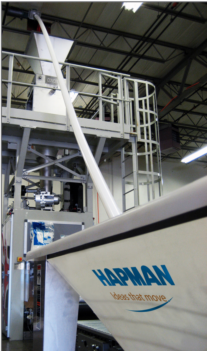
Hapman's 300 Series Helix flexible screw conveyor with polyurethane hopper and flat wire auger conveys plastic pellets 28 feet (8.5 meters) to the TB 1200 form-fill-seal solution.
